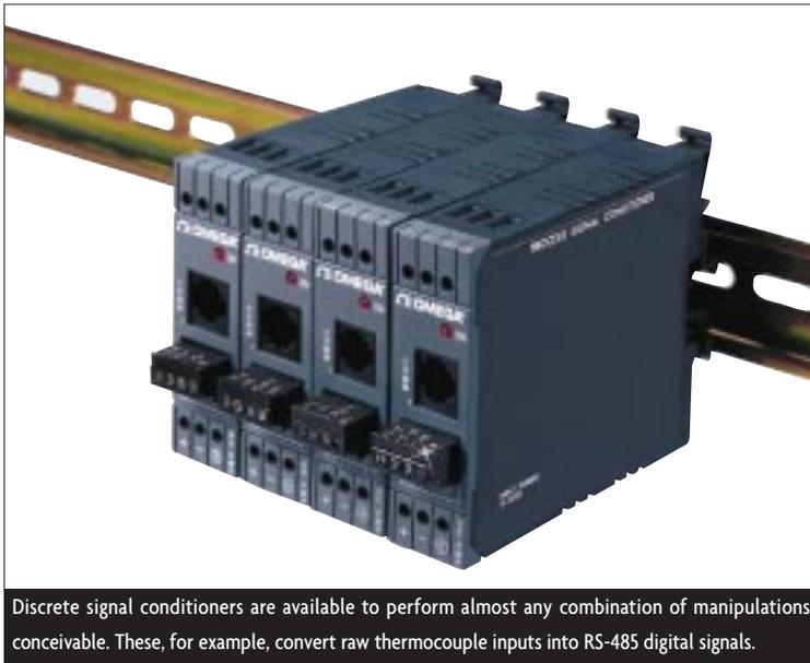
Discrete signal conditioners are available to perform almost any combination of manipulations conceivable. These, for example, convert raw thermocouple inputs into RS-485 digital signals.
