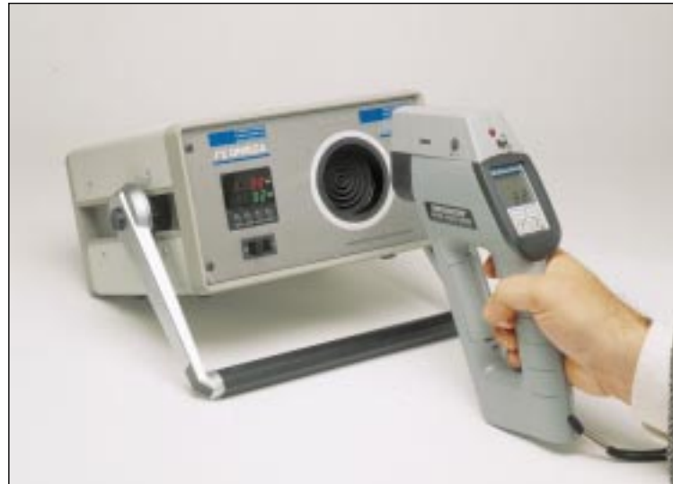
A handheld IR thermometer is calibrated against a commercial blackbody source—the internal cavity is designed to closely approach a blackbody's unity emissivity.
